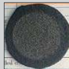
After abrasion test >8000 cycles without breaking the material
