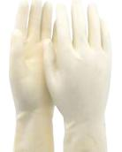
Chemical protection glove in specially formulated latex rubber. Dust free exterior and interior surface. Surface treated. Unlined. Food handling approved. Silicone free. Length (mm): 295 +/- 10, Weight (g): 0.52 +/- 0.02
