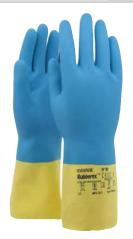
Chemical protection glove in triple layer rubber. Slightly thicker for greater abrasion and chemical resistance, primarily against oils and fats. Excellent grip in both wet and oily conditions. Cotton flocklined interior for comfort. Food handling approved. Silicone free. Length (mm): 320 +/- 10, Thickness (mm): 0.7 +/- 0.03
