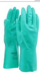
Chemical protection glove in nitrile rubber with excellent resistance against oils, fats, aromatic and petrolum based chemicals. Raised diamond pattern in the palm for increased grip in both wet and oily environments. Cotton flocklined interior for comfort. Food handling approved. Silicone free. Length (mm): 315 +/- 10, Thickness (mm): 0.38 +/- 0.03
