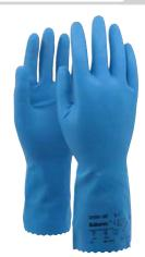
compound for better oil and fat resistance. Excellent grip in both wet and oily conditions. Satin lined interior for maximum comfort. Food handling approved. Silicone free. Length (mm): 300 +/- 10, Thickness (mm): 0.50 +/- 0.05
