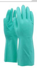
Chemical protection glove in premium grade nitrile rubber with excellent resistance against fats, aromatic and petrolum based chemicals. Raised diamond pattern in the palm for increased grip in both wet and oily environments. Dust free exterior and interior surface. Unlined. Food handling approved. Silicone free. Length (mm): 330 +/- 10, Thickness (mm): 0.40 +/- 0.03
