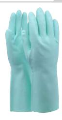
Light but still durable chemical protection glove in specially formulated nitrile rubber. Excellent resistance against fats, oils and detergents. Very good grip in both wet and oily environments. Exceptionally comfortable and flexible glove with cotton flocklined interior for comfort. Food handling approved. Silicone free. Length (mm): 330 +/- 10, Thickness (mm): 0.28 +/- 0.03
