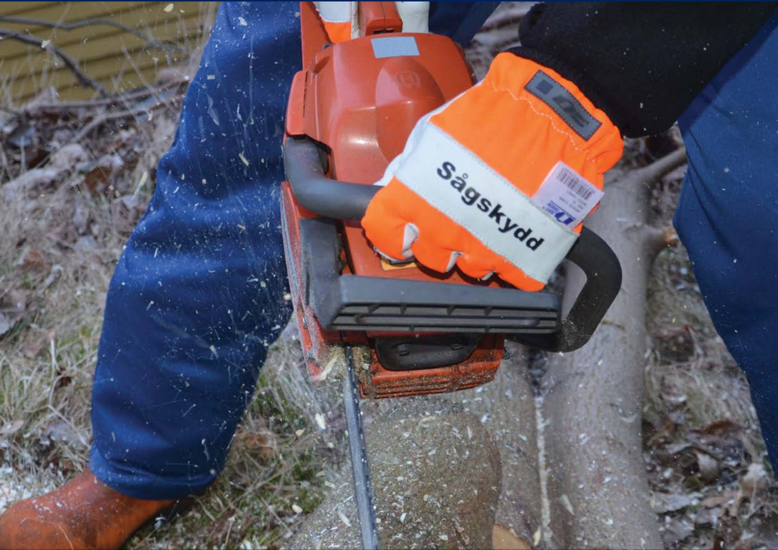
Chainsaw protection gloves - with ballistic nylon fibres
